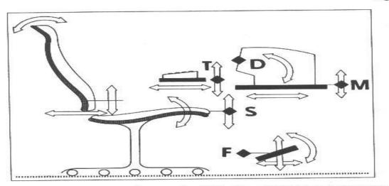
Figure 10-4. Adjustment features of a VDT office workstation. Key: S = seat height; T = table; F = footrest; D = monitor; M = support. (Reprinted with permission from Kroemer, 1985.)
